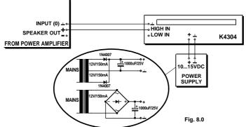
Connect the unit to a suitable supply voltage between 10VDC and 15VDC, this can also be a standard DC adapter. You can also build your own power supply, see diagram. Use a 2x12V transformer, two rectifier diodes and a electrolytic capacitor or use a single 12V transformer with a bridge rectifier and a electrolytic capacitor.
