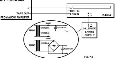
Connect the unit to a suitable supply voltage between 10VDC and 15VDC, this can also be a standard DC adapter. You can also build your own power supply, see diagram. Use a 2x12V transformer, two rectifier diodes and a electrolytic capacitor or use a single 12V transformer with a bridge rectifier and a electrolytic capacitor.
