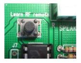
Keep push button SW13 pressed while transmitting with the remote. The LCD display will blink twice to confirm that the remote is learnt (if no display is mounted LED LD4 will blink twice).
