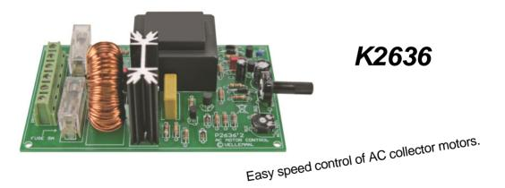
This kit is especially designed to control the speed of drills or any other AC-motors with carbon brushes. Contrary to the usual dimmers, there isn't a phase cut every 1/2 period but only once per period. The moment of cutting determines the speed which can be adjusted from 5 to about 95 %. Owing to this kind of controling, we keep a higher torque at low speed. This does not mean on the other hand, that this circuit cannot be used for a resistive load (e.g. lamps, heating devices.).
